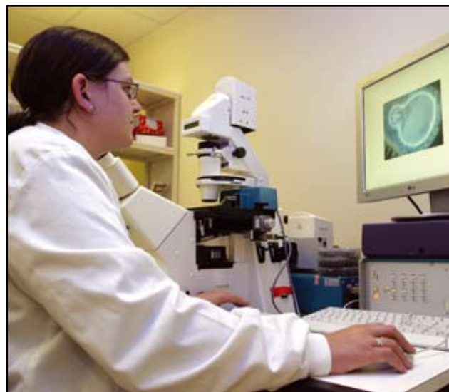
The new laser cell capture microscope. Julie Christie prepares to "cut and paste" material with microscopic precision.
