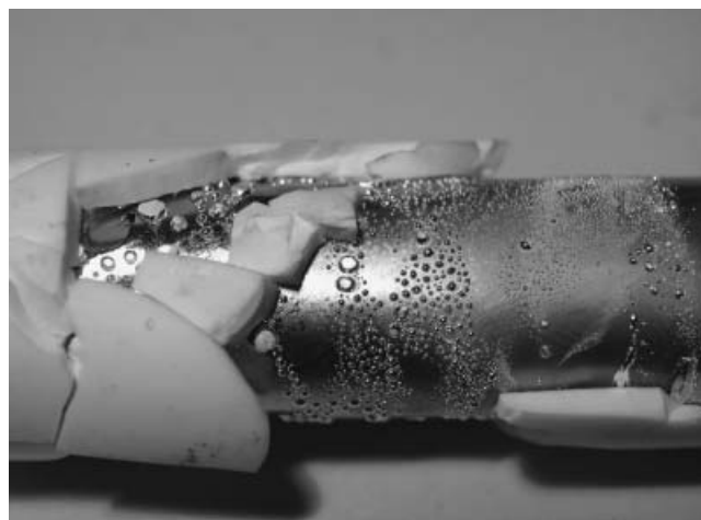
Figure 10. Molybdenum tube after 8 weeks and 700 samples. The top of the tube is to the left, with the top of the hotspot at the right. The alumina tube was shattered with a hammer and fragments of alumina are cemented to the molybdenum with silver. Larger drops of silver at the left may be associated with pin-holes, the smaller droplets at the right show surface diffusion from right to left, to the cooler end of the tube.
